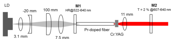
Fig. 7 Experimental setup of passively Q-switched Pr-doped fiber laser by utilizing a Cr 4+ :YAG saturable absorber
