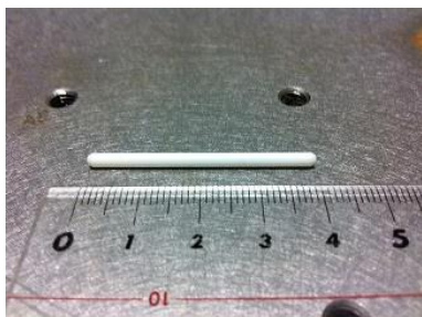
Fig. 2 Photograph of the employed Pr-doped fluoride fiber fabricated by Sumita Optical Glass Inc.
